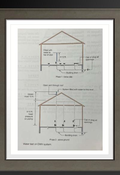
• The head pressure for a water test of drain, waste and vent system has been increased from 5' to 10'. Air vacuum testing is now permitted for plastic piping is DWV.
