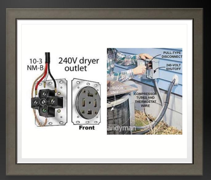
OUTLET. A point on the wiring system at which current is taken to supply utilization equipment. **RECEPTACLE.** A receptacle is a contact device installed at the outlet for the connection of an attachment plug. A single receptacle is a single contact device with no other contact device on the same yoke. A multiple receptacle is two or more contact devices on the same yoke. **RECEPTACLE OUTLET.** An outlet where one or more receptacles are installed.
