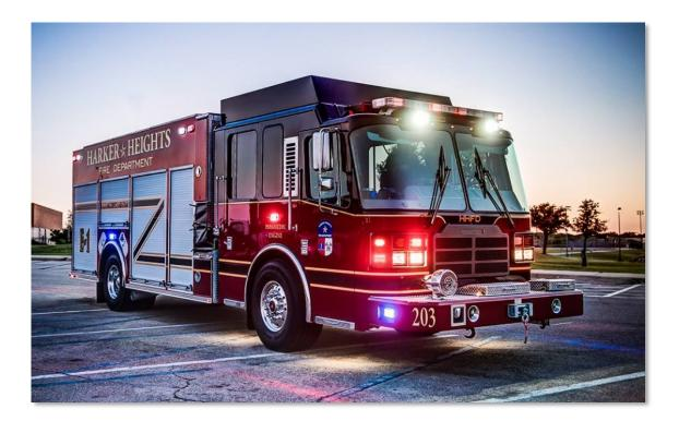
Engine 1 is a 2014 Ferrara MVP Pumper Truck. It can store up to 750 gallons of water and pump 2000 gallons per minute. It carries up to 768 cubic feet of equipment. The truck is approximately 34' long and 10' in height.
