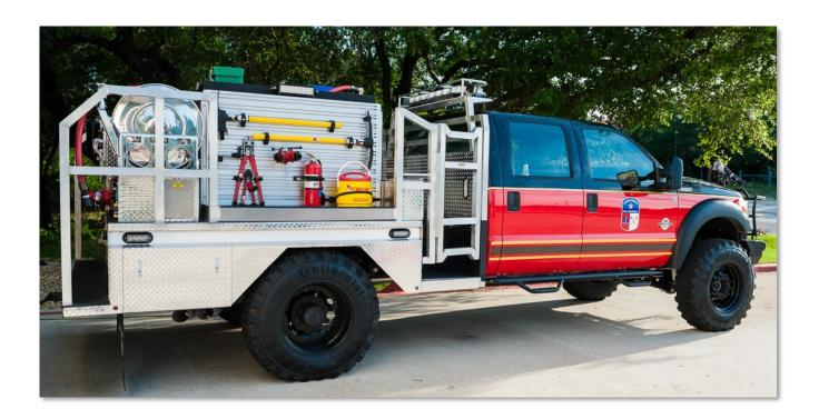
Brush Trucks are designed to move quickly through areas that other fire apparatuses cannot. They can store up to 400 gallons of water and can be used for light rescue, initial attack or medical support. Our trucks are also equipped with a remote controlled nozzle, which enables the vehicle to fight fire while on the move.
