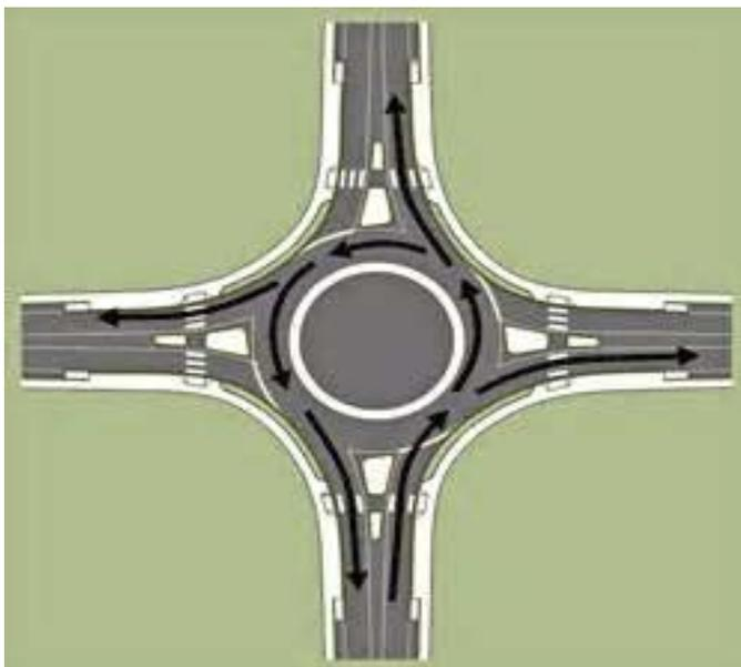
Although the picture to the left is not the design for Commercial Drive, it provides an idea of what a roundabout is and how it functions for traffic flow.
