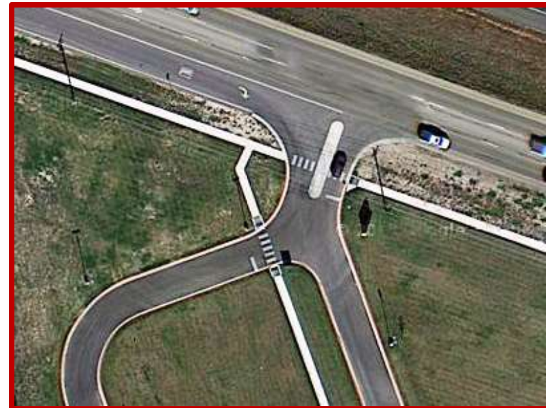
Figure 19 - Sidewalk Markings Extended Across a Driveway
